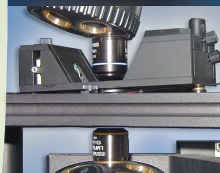
▲ MultiView 1000™ Head integrated with a standard microscope
